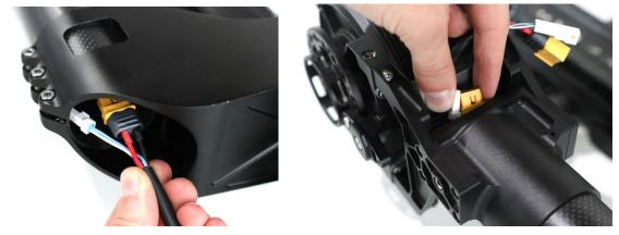
**Step 11)** Reconnect the Tilt ESC power and data cables, then carefully route them back into the tube, and replace the Tilt ESC cable guard.
