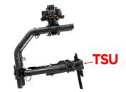
Step 2) Remove the 4 screws securing the TSU cover, and remove the TSU cover.
