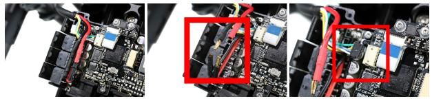
**Step 4)** Remove the front foam plug from the passive carbon fiber Roll arm, then remove the rear foam plug and **carefully** feed the TSU cable back through the Roll arm, finally remove the center carbon fiber plate to pull the TSU cable through the Roll arm (Cable should stay routed through the Roll motor.)
