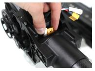
Step 9) Remove the rear foam plug and route the Tilt ESC Cable back through the aluminum Roll arm.
