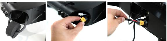
**Step 10)** Just like TSU Cable, route the Tilt ESC under or over (whichever is less likely to snag) the aluminum Roll arm, and then into the carbon fiber tube, and finally up through gap between the ESC and the mount.
