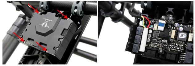
**Step 3)** Remove the white heat shield, disconnect the red and black bullet connectors, then **carefully** remove the small black data connector from the white receptacle to free the TSU Cable.
