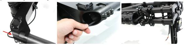
**Step 6)** Reconnect the black data connector, reconnect the red and black bullet connectors, replace the heat shield, and finally replace the cover using the 4 fasteners originally removed. Make sure no cables get snagged or damaged, and check that all rubber connector covers can be properly seated around the perimeter of the TSU cover.
