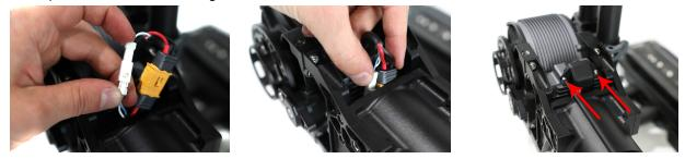
Step 12) Remove both rear Roll arm stopper screws, and loosen the 6 Roll arm clamp fasteners.
