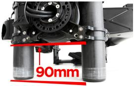
**Step 3)** Finally, re-tighten the 2 bolts on the GCU Mount, and the 4 bolts on the Roll Motor Mount (6 total). Even with the addition of the M6 Standoffs for the Passive Plates, we've reduced the pendulum length of the camera package by almost 2 inches.
