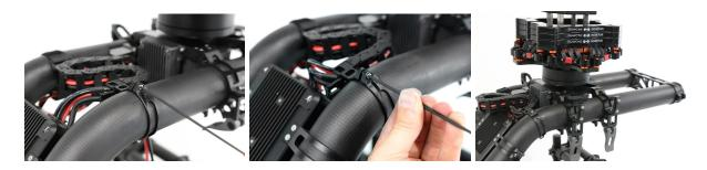
**Step 15)** Ensure that all fasteners have been re-tightened, cables have been properly routed and connected, and the camera package is free to rotate without resistance of interference.
