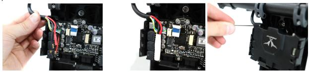
**Step 7)** Disconnect the cable guard from the Tilt Motor ESC, then carefully lift the power and data cables up through the gap between the ESC and the mount.
