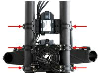
Step 2) Slide the GCU Mount and Roll Motor Mount Upwards on the XL spine ~90mm. Make sure your camera package can still look +/- 90° freely without making contact with the XL spine or pan motor. If more room is needed, slide the GCU and Roll Motor Mount downwards on the XL spine.
