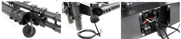
**Step 5)** Rather than feeding the TSU Cable back through the aluminum Roll arm, route the cable under or over (whichever is less likely to snag) the aluminum Roll arm, and then into the carbon fiber tube, and finally back through the Tilt cage down to the TSU.
