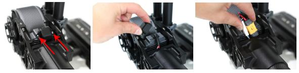
Step 8) Carefully disconnect the Tilt power and data cables, and push them back down into the CF tube.
