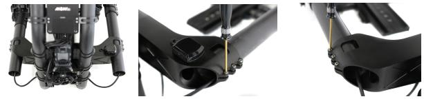
**Step 14)** Loosen the Pan Motor cable guide clamp, and slide it back, this will make room for the Pan Motor to slide further back for balancing.
