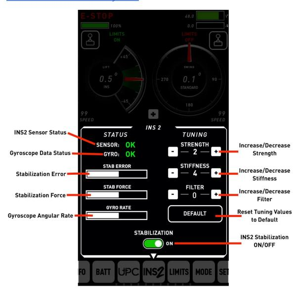
**STRENGTH**- Controls the magnitude of the correction applied to the Lift axis based on position error – maintains target angle of the Boom.
