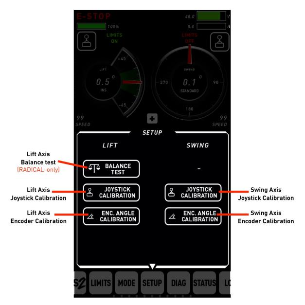
**Balance Test**- Helps to detect any Lift Axis imbalance between payload and counterweight by eliminating the electromotive torque present in a gear-reduced powertrain.
