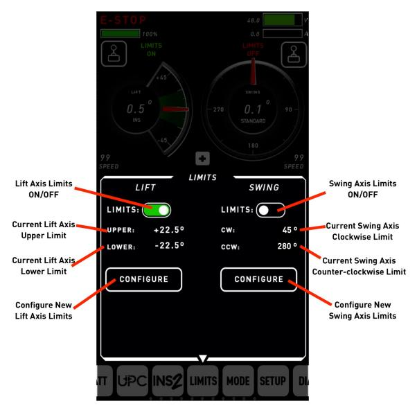
**Limits ON/OFF**- Toggles range of motion for that axis on or off. When Limits are turned off, previous Limit values are stored. If Limits are turned ON when the arm is not within the specified range, the arm will move freely until it is within range, then no longer move beyond the limits.
