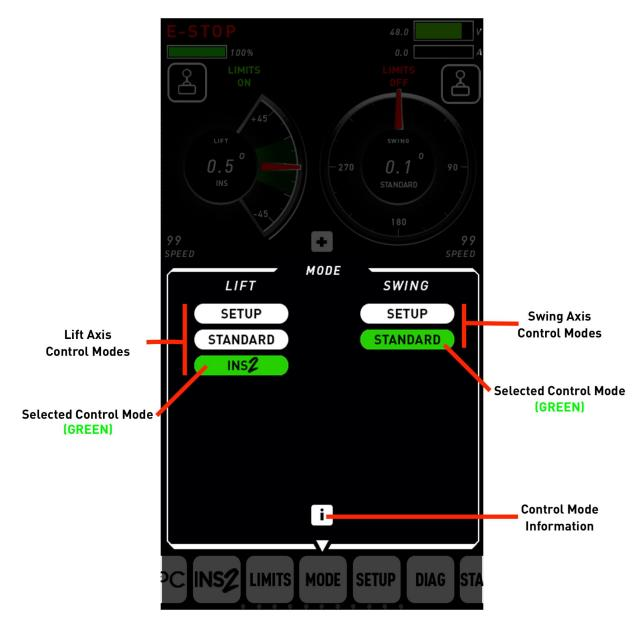
**SETUP Mode**- This mode is used for during physical setup or bench-testing, when no payloads are attached. Because this is an open-loop Control Mode, Limits are not available in this Control Mode. **STANDARD Mode**- Uses encoder data for closed-loop position of the axis. Recommended for normal operation if INS is not available.
