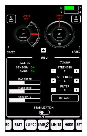
Within the RADICAL INS 2 Control Panel, there is a STATUS section, Performance Monitoring Gauges and adjustable TUNING parameters
