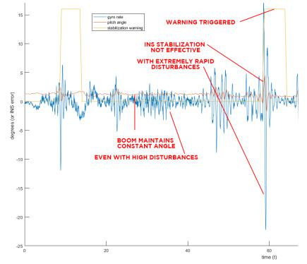
In the figure above, the orange line represents the Lift Axis (boom) angle, the blue line represents the gyro rate, and the yellow line represents the warning that the vehicle is driving in conditions where stabilization is not as effective. Notice at the :58 second mark, the RADICAL INS 2 warning is triggered, alerting the operator that incoming disturbance has surpassed what the RADICAL INS 2 tuning is capable of.
