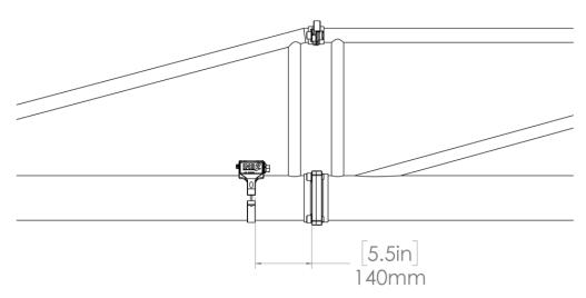
2. Fasten the unit to the boom using the provided M4 fasteners - make sure the top of the housing is horizontal (this is not *critical*, but the more accurate it is, the better the performance will be - visual alignment should be sufficient)
