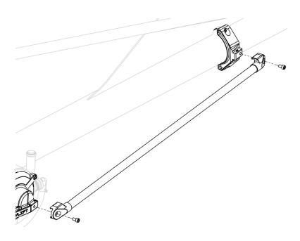
5. Attach the End Brace to the L/S Kit Lateral Brace and End Brace Boom Mount using 2x SHCS M8. Apply appropriate torque to the fasteners.
