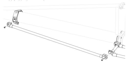
9. Repeat steps 4, 5, 6, 7 & 8 on the other side of the booms. **Loosen the mounts to make slight adjustments if necessary.** Make sure the braces are centered, and are not crooked. After adjustments have been made, ensure all fasteners are properly tightened.
