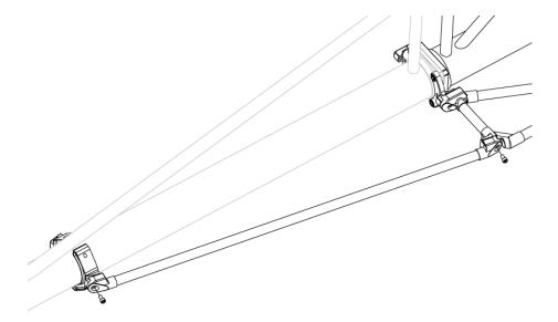
6. Repeat step 3, 4, & 5 on the other side. **Loosen the mounts to make slight adjustments if necessary.** Make sure the braces are centered, and are not crooked. After adjustments have been made, ensure all fasteners are properly tightened.
