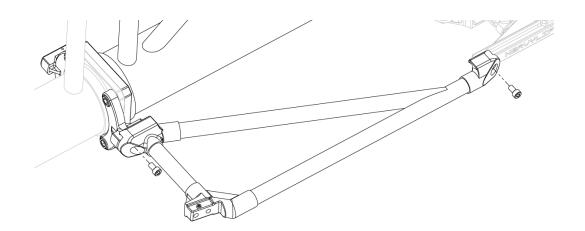
4. Attach an End Brace to the Passive Mount and End Brace Boom Mount using 2x SHCS M8. Apply appropriate torque to the fasteners.
