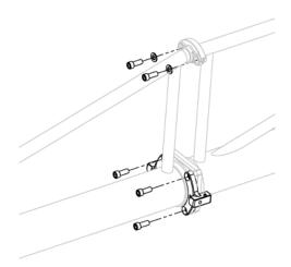
4. Attach a L/S Kit Lateral Brace to the Passive Mount and Center Brace Boom Mount using 2X SHCS M8. Make sure the clip receivers are hooked over the SHCS M4 fastener heads before letting go. Apply appropriate torque to the fasteners.
