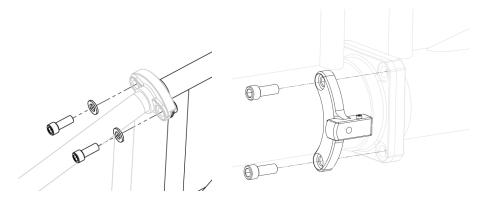
3. Attach a L/S Kit Lateral Brace to the Passive Mount and Center Brace Boom Mount using 2X SHCS M8. Make sure the clip receivers are hooked over the SHCS M4 fastener heads before letting go. Apply appropriate torque to the fasteners.
