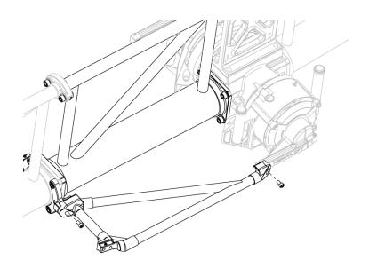
5. Install an L/S Kit 14' Mode adapter to the L/S Kit Lateral Brace using 2X SHCS M8, and apply appropriate torque to the fasteners.
