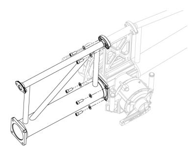
2. Install the Front Boom to the L/S Kit boom by securing the clip receiver. Install the x2 SHCS M12 fasteners to the top flange of the boom and then install both Center Brace Boom Mounts to the Front Boom plate using 2X SHCS M12 on each side. Apply appropriate torque to the fasteners.
