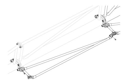
7. Attach an End Brace to the Passive Mount and End Brace Boom Mount using 2x SHCS M8. Apply appropriate torque to the fasteners.
