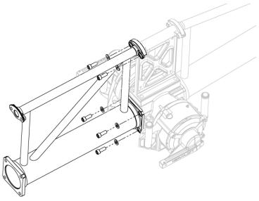
2. Install the Middle Boom to the L/S Kit boom by securing the clip receiver. Install the x2 SHCS M12 fasteners to the top flange of the boom and then install both Center Brace Boom Mounts to the Middle Boom plate using 2X SHCS M12 on each side. Apply appropriate torque to the fasteners.
