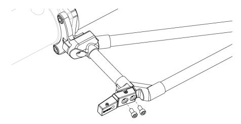
6. Install a Heavylift Center Brace to the L/S Kit Adapter and Center Brace Boom Mount using 2X SHCS M8. Apply appropriate torque to the fasteners.
