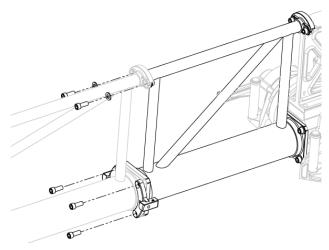
3. Install the Front Boom to the Middle Boom by securing the clip receiver over the Middle Boom clip. Install the x2 SHCS M12 fasteners to the top flange of the boom and then install both Center Brace Boom Mounts to the Front Boom plate using 2X SHCS M12 on each side. Apply appropriate torque to the fasteners
