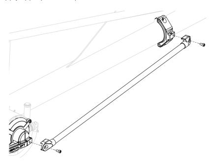
8. Attach an End Brace to the Center Brace and End Brace Boom Mount using 2x SHCS M8. Apply appropriate torque to the fasteners.
